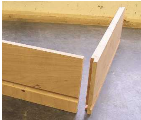
▲ Pic.17 The drawers were constructed with simple half lap joints...
